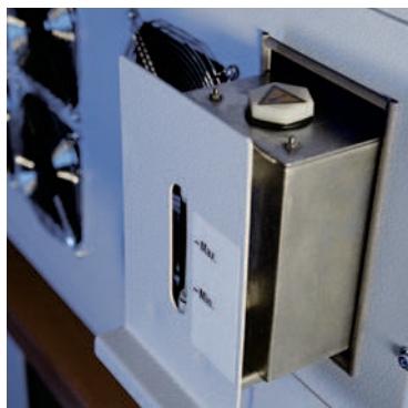
Internal water chiller
