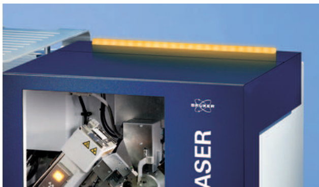
X-ray warning lights
