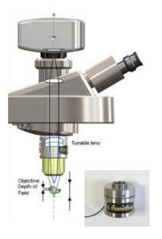
Instead of moving the sample to perform Z-plane scanning, the specimen is set in a fixed position while the illumination and the detection planes simultaneously move through the sample. The sample remains in a steady position, minimizing vibrations and perturbation issues. The illumination plane is scanned using a galvanometric mirror, while the detection plane is scanned using a remote focusing device to provide high-speed, perturbationfree 3D imaging at 75 images/second.
