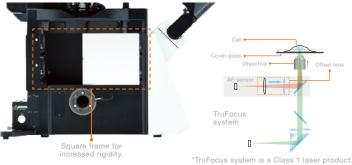
The square frame architecture and focus drive design of the IXplore™ system enhance rigidity and reduce the impact of vibration and temperature. This design, combined with our TruFocus™ system, facilitates reliable time-lapse imaging by maintaining the desired position along the Z axis.
