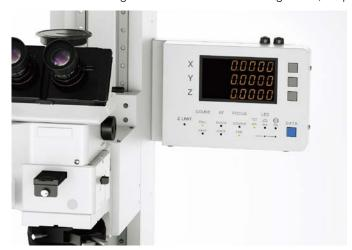
Digital readout attached to the frame
